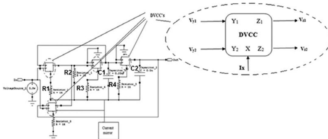
**Fig.4 DVCC and passive components connections**
