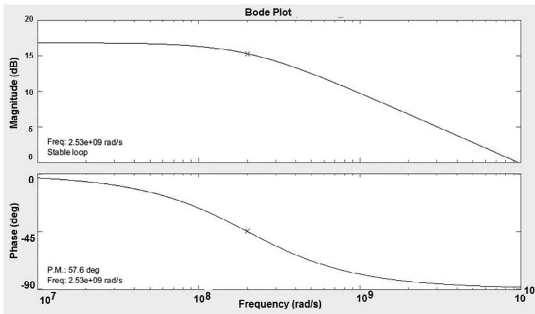
**Fig.6 Bode plot of transfer function**
