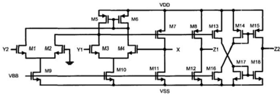
**Fig2. Circuit diagram of CMOS based DVCC**
