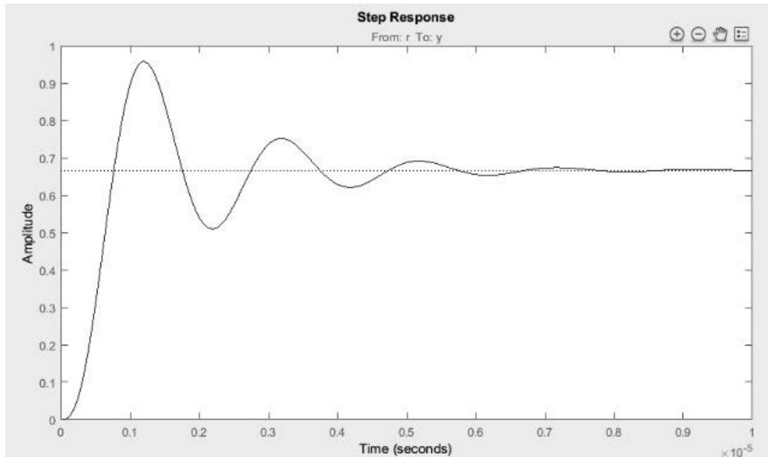
**Fig.5 Step response of transfer function**
